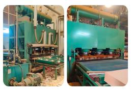
**Short Cycle Lamination Presses** For paper lamination on particle board, MDF, and wooden flooring.
